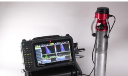
With its modular design and internally built encoder this scanner can be utilised in multiple configurations whilst remaining robust and suitable for extensive in-field operation.
