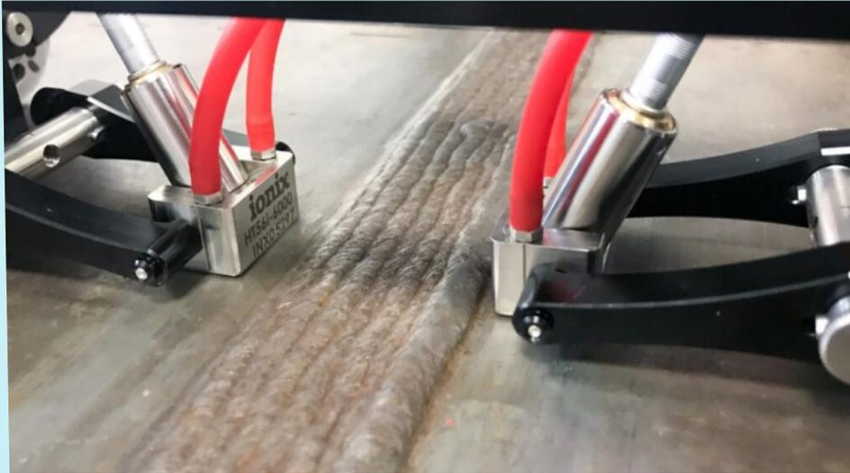
Ultrasonic time-of-flight diffraction (TOFD) is a popular method widely used in petrochemical, energy and other industries for the in-service detection and characterisation of weld defects such as root corrosion, porosity, inclusions, and cracks. However, with increasing demand for on-stream measurements, conventional TOFD is limited due to the temperature at which these probes can operate, often causing failure of the transducer, or causing noise in the wedges to mask the ultrasound signal.....
