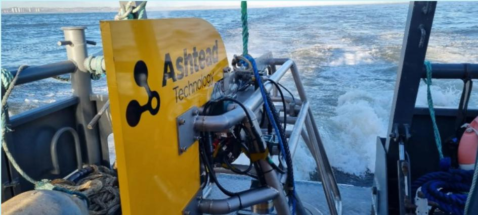
Ashtead Technology has launched its new standard drop camera system, part of a range of systems designed for high-resolution seabed visual inspection, in water depths down to 4000m.
