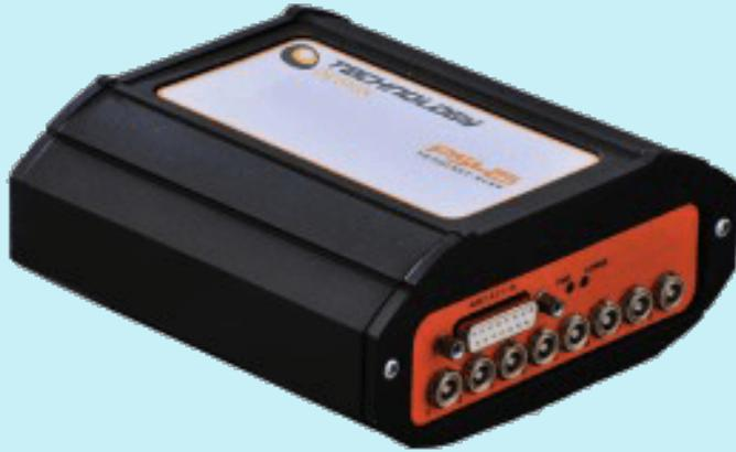
The Ethernet connection simplifies the link between laptop and Pocket-Scan and eliminates the need for a PCMCIA type II card slot. The Ethernet system requires minimal initial setup with no special drivers and will communicate with any Ethernet enabled PC.
