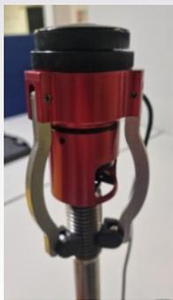
This multi-purpose modular scanner is capable of scanning 1" to 3" studs and surface scanning circumference up to 400 mm diameter. The modular design allows the scanner to be reconfigured with various probe holders, switchable magnet, and face scanning arm.
