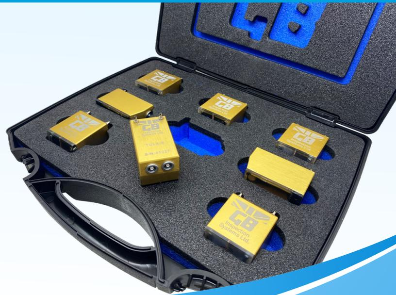
The TULA (TOFD Ultra Low Angle) range of transducers were developed for the early stage detection of HTHA in material ~25mm thick, we are now pleased to announce that the range has been extended.
